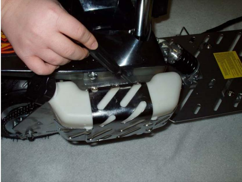
**Attach the gas lines to the engine.**
