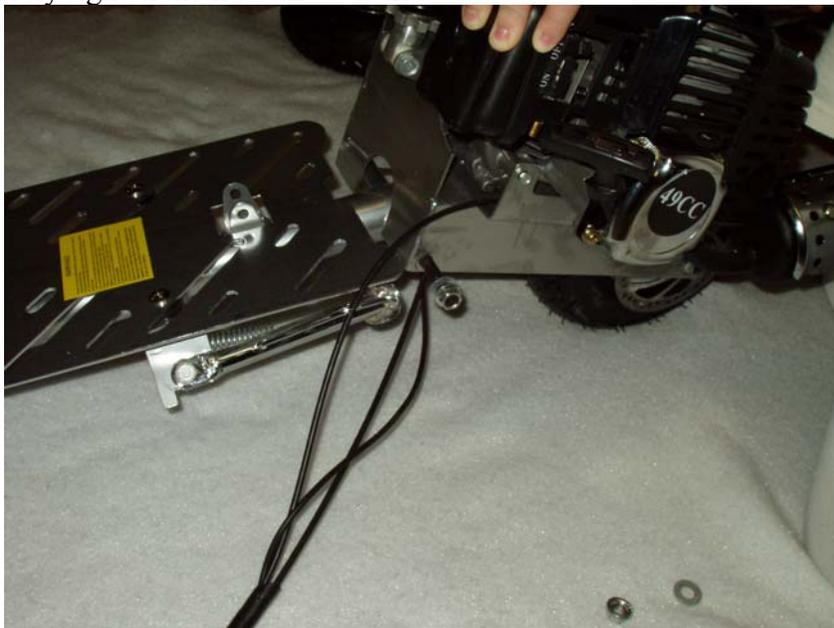
**Attach the rear mono shock to the front frame.**
