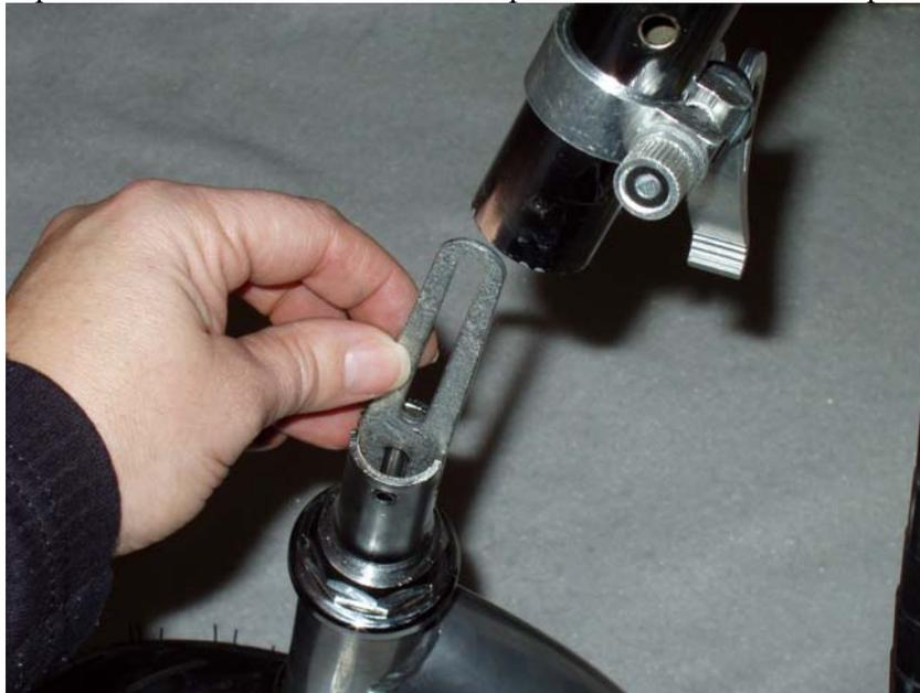
Align the handlebars correctly and then re-insert the pin bolt and screw into the handlebar post. This will keep the handlebars in line with the wheel. Tighten the clamp securely.
