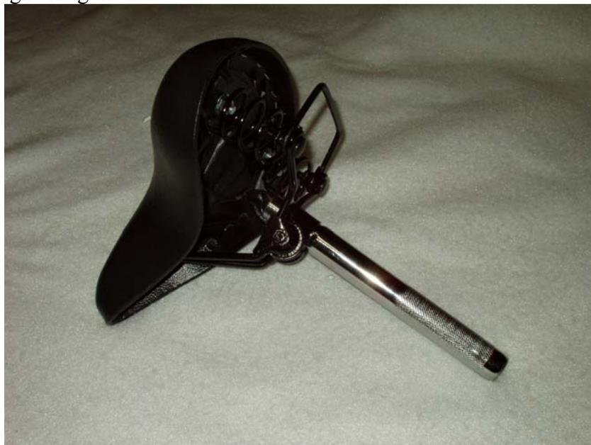
The second seat post is inserted into the opening on the rear/motor frame. Tighten the post in place by using the enclosed allen wrench.
